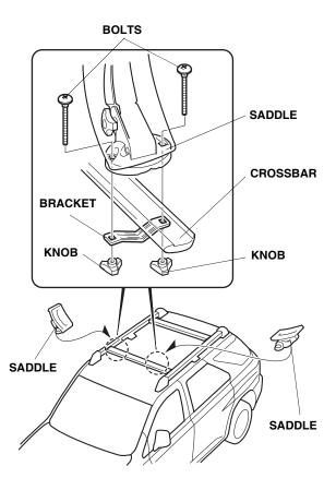
Position the two hydro-glide assemblies on the rear crossbar, and loosely install the hydro-glide assemblies using one bracket, two bolts and two knobs for each assembly. The distance between the two assemblies should be the same width as the kayak.
