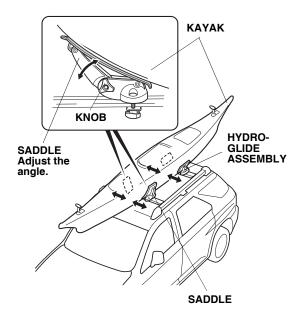
5. Slide the kayak forward or backward until it's level with the roof. If necessary, loosen the knob on each saddle and adjust the saddle angle to fit snugly against the kayak. Tighten each knob securely.
